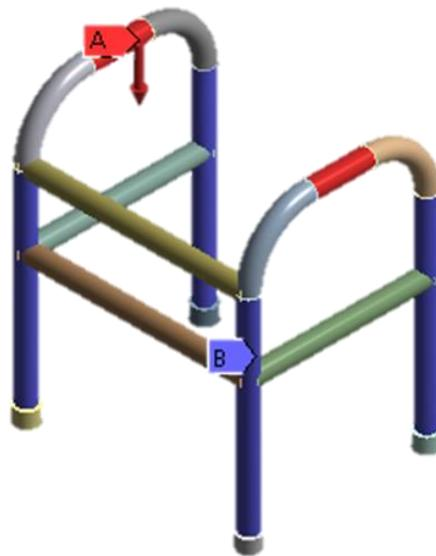
**Figure 2.** Boundary condition of static structural simulation of walker
