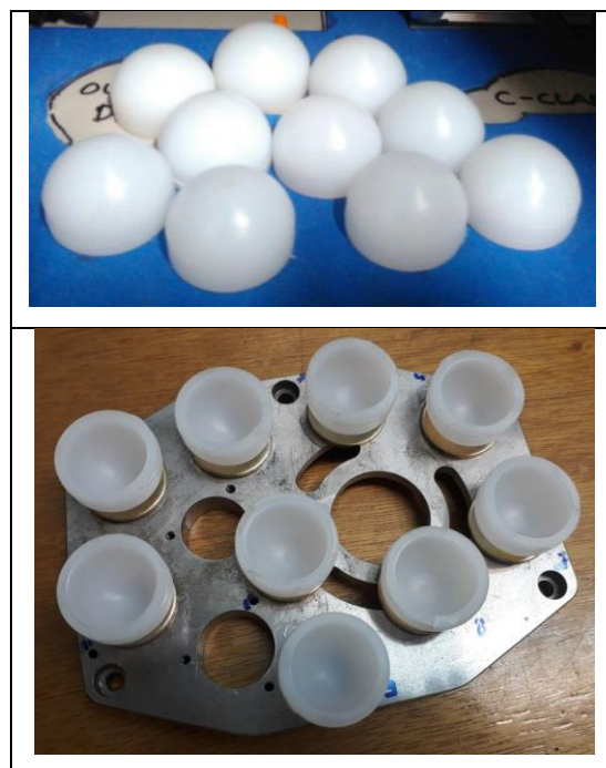
Figure 2. Acetabular Liner UHMWPE result from CNC milling
