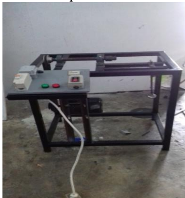
Gambar 1 Mesin Uji Fatik Tipe ( cantilever rotary bending )
